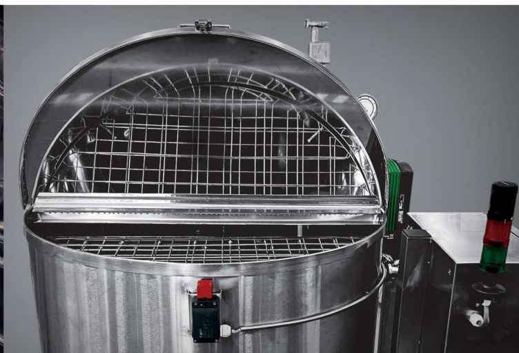
Bottle unloading grid
